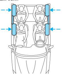
The Safety Canopy<sup>®</sup> system, in combination with safety belts, can help reduce the risk of severe injuries in the event of a significant side impact collision or rollover event.
